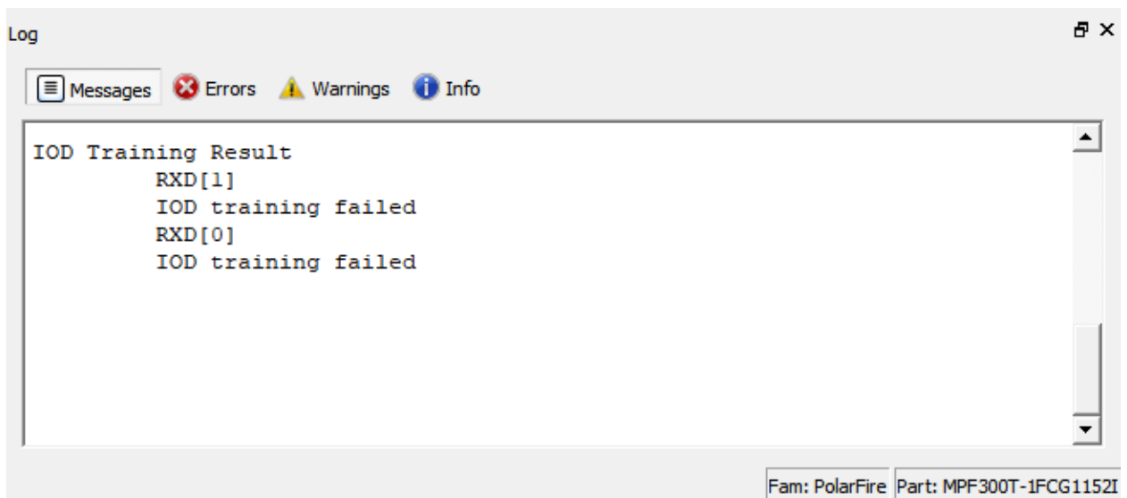
Figure 3-94. SmartDebug Log Window—Training Failed
